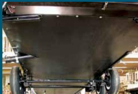
*The enclosed underbelly eliminates turbulence caused by exposed frame members, holding tanks, plumbing etc.*
