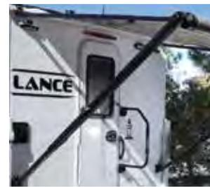
Rear Awning - Provides protection from the elements over the rear of your camper. Is model specific in either electric or manual operation. N/A 1172
