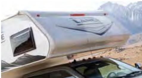
TPO Front Nose Cap - Protects your camper from debris and leaks while reducing drag and increasing fuel economy.
