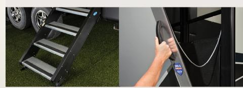
MORryde® Step Above™ Safe and secure main entry with strut assist.
