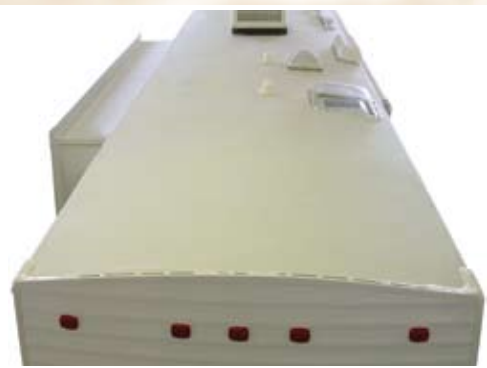
3/8" crowned truss, walk on roof decking.
