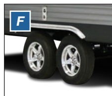
F CATALINA'S EXCLUSIVE TIRE AND RIM PACKAGE INCLUDES: RADIAL TIRES, POLISHED ALUMINUM FENDER SKIRTS AND E-COAT MAINTENANCE FREE RIMS
