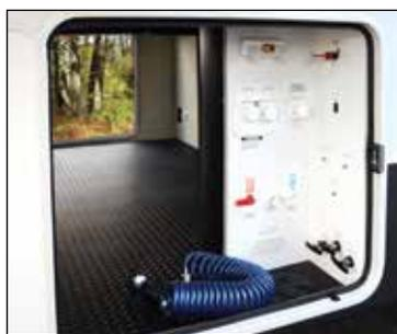
The newly updated fully enclosed and LED lighted docking center includes a removable coiled hose outside shower, black tank flush, winterization kit, water heater bypass, battery disconnect, and dedicated cable and satellite jacks.
