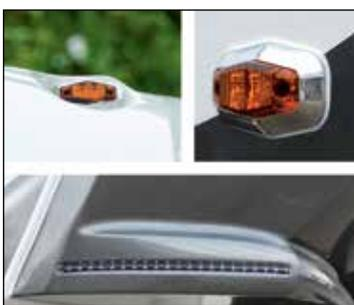
Low power, high impact exterior LED lighting is both highly visible and energy efficient. All of Wildcat's interior lighting is LED as well!
