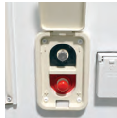
Remote Charging Port makes charging batteries easier.
