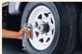
Jay Flight's E-Z Lube™ axles with removable caps make maintenance a snap. (G2 models only)
