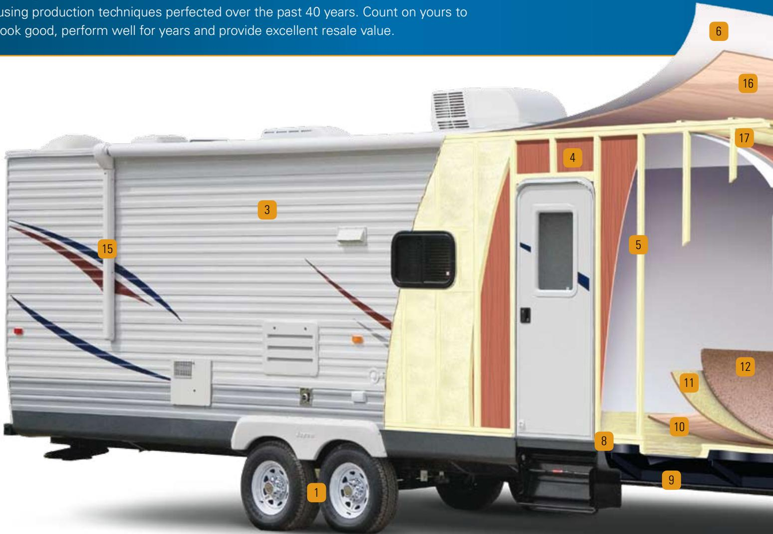
1. Jay Flight's E-Z Lube® axles with removable caps make maintenance a snap (G2 models only)
