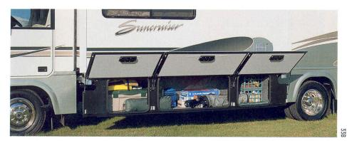
Cas struts (on most doors) and single paddle latches allow easy, one-handed opening of the large storage bays. For easy access and a lighter keychain, Suncruiser features the Tri/Mark KeyOne™ System that incorporates common-key locks for the main entry door, driver's door, storage compartments and fuel fill. And thanks to our revolutionary STOREMORE™ technology, all basement compartments feature full-size openings — even under the slideout.
