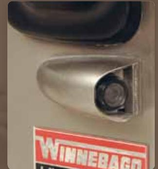
**Sideview Cameras** Sideview cameras activate with the turn signals and provide an added sense of comfort when maneuvering.
