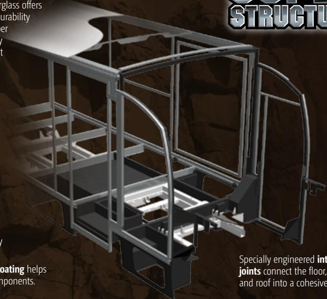
Specially engineered **interlocking joints** connect the floor, sidewalls and roof into a cohesive unit.
