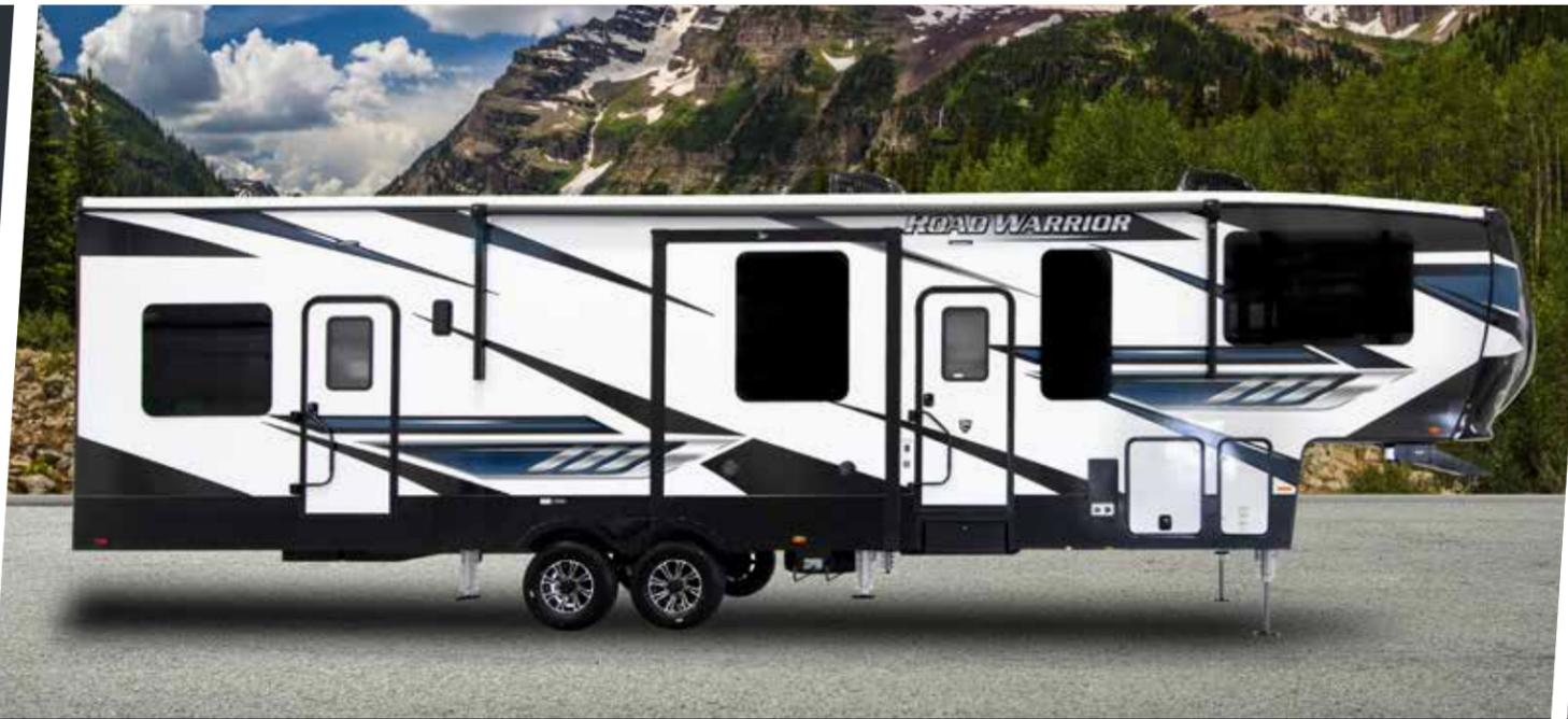
All Road Warrior units are proudly crafted with Azdel composite sidewalls. Half the weight of wood, environmentally friendly panels lighten your load while increasing your trailer's durability and insulation value. Azdel also resists water, sound and temperature changes, keeping your living spaces comfortable and quiet.
