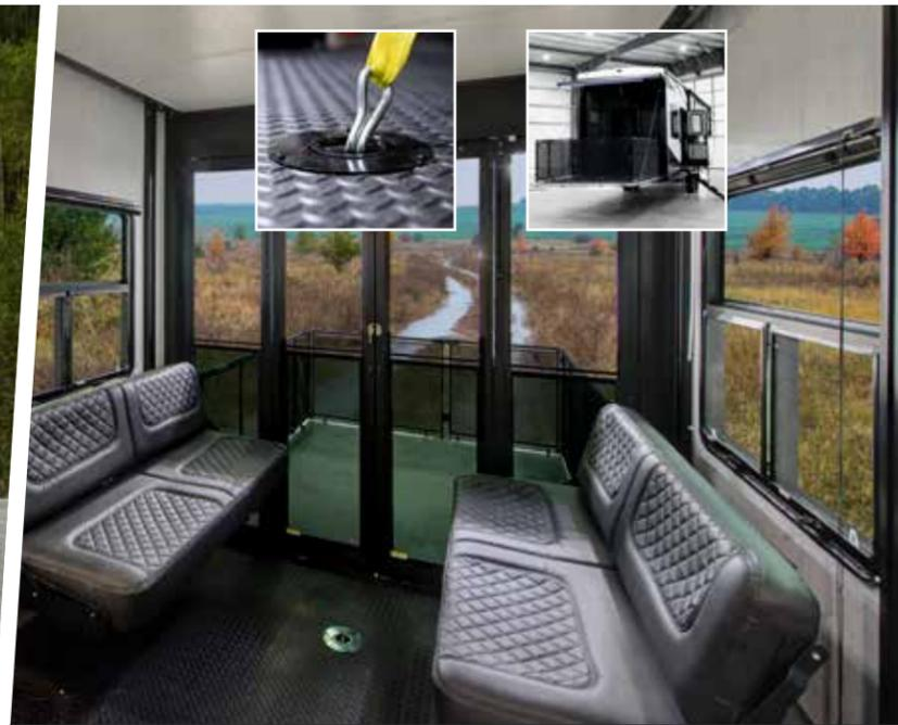
New Zero-Gravity ramp door is designed to easily raise or lower with no resistance and provide easy access to your gear with the lift of a finger. Also new is the frame-welded tie down system, each one supporting up to 5,000lbs.
