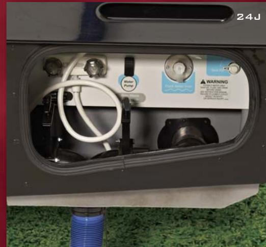
**EXTERIOR SERVICE CENTERS** The exterior service centers house water, drainage facilities and the available exterior wash station. Electrical hookups can also be found here, including a power cord with the QuickPort® service connection hatch (Not available on 24J shown here). This hatch allows you to close the compartment door even when connected to hookups at the campground.
