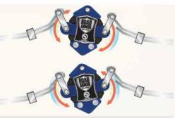
Road Armor™ Suspension w/ 360° Vibration Control Equalizes axle load to dampen shock and vibration. (TrailAir on 380/381TH models.)
