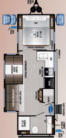
DRY HITCH (LBS.): 775 UJVW (LBS.): 6,473 CGG (LBS.): 3,102 LENGTH W/HITCH: 30' 6" EXTERIOR HEIGHT: 11' 2" WIDTH: 96" TANKS (F/G/B): 40 / 60 / 30 AWNING: 15'
