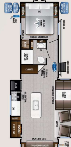
DRY HITCH (LBS.): 1,063 UJVW (LBS.): 7,407 CGG (LBS.): 2,456 LENGTH W/HITCH: 36' 1" EXTERIOR HEIGHT: 11' 3" WIDTH: 96" TANKS (F/G/B): 40 / 60 / 30 AWNING: 11'
