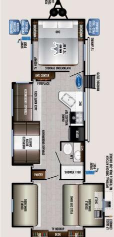
DRY HITCH (LBS.): 996 UJVW (LBS.): 8,745 CGG (LBS.): 2,951 LENGTH W/HITCH: 37' 5" EXTERIOR HEIGHT: 11' 3" WIDTH: 96" TANKS (F/G/B): 40 / 60 / 30 AWNING: 15'
