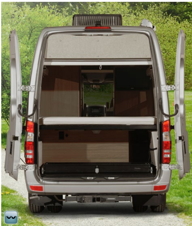
The Rear Double Doors open up to 270 degrees revealing a slideout storage tray (70A).
