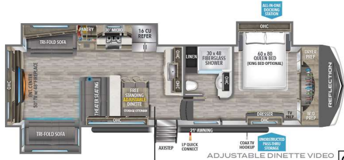
341RDS U 1 V 1 W 1 10,964 HITCH 1 2,072 LENGTH 2 36' 11" HEIGHT 3 12' 6" CAPACITY 74 87 47
