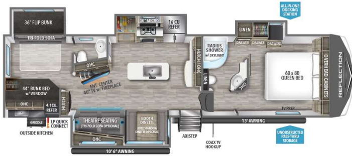
311BHS U 1 V 1 W 1 11,377 HITCH 1 2,316 LENGTH 2 36' 10" HEIGHT 3 12' 3" CAPACITY 74 87 87
