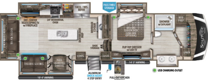
372WB 372WB-R U VW ' HITCH' GVWR LENGTH' HEIGHT CAPACITY 13,950 2,800 16,800 41' 4" 13' 5" 93 100 50
