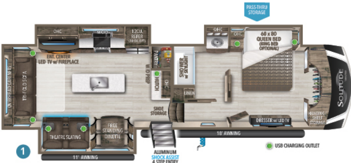
3540GK 3540GK-R U/VW 1 HITCH 1 GVWR LENGTH 1 HEIGHT CAPACITY 12,758 2,544 16,800 38' 3" 13' 5" 91 100 53
